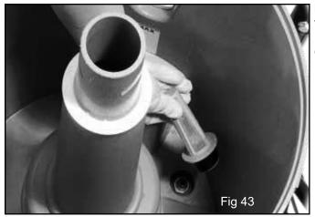
Located in the bottom of the NuChem / water tank is a barrel filter (Fig 43).
