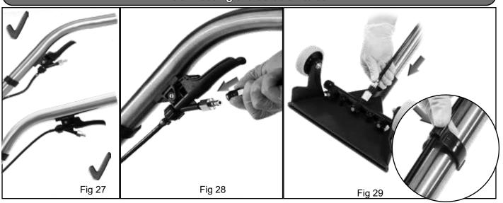
The solution tube has been designed so the trigger can be fitted either way on to the stainless curved wand. (fig 27)
