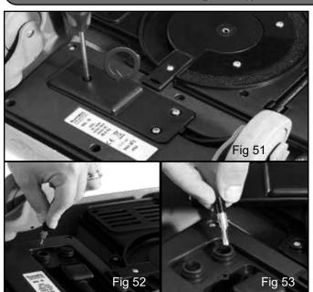
Under the rectangular plate is 6.3 amp time lag fuse holder Remove the plate (Fig 51).
