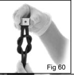
Fit the new cable to the strain relief (fig 60) and refiit to the machine (fig 61).
