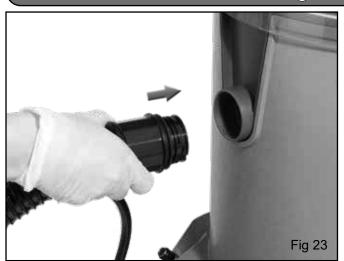
Fit the Vacuum hose to the front of the machine (Fig 23).
