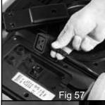
Lift the cable off the pins (fig 57) and remove from the plastic clips (fig 58).
