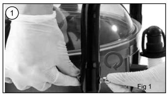
Fit the handle to the machine using the fixings supplied. (Fig 1)
