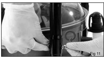
Secure the handle using the nut and bolt supplied (Fig 11).
