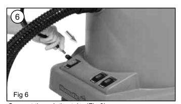
Connect the solution tube (Fig 6)
